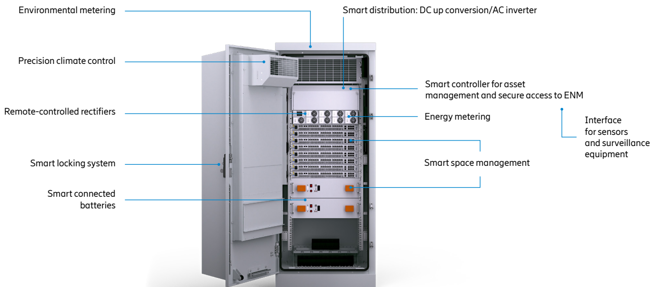
Figure 10: An overview of Ericsson Smart Connected Site
